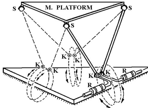
Fig. 1. The 6-RKS parallel manipulator introduced by Hunt.
