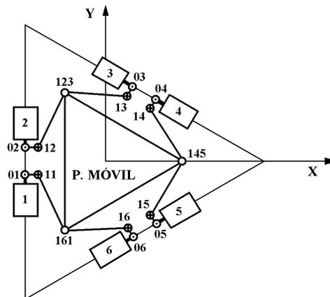
Fig. 2. Notation used to describe the parallel manipulator.
