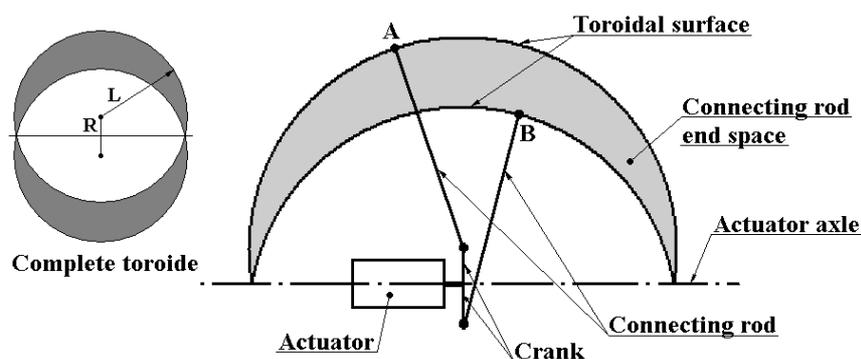
Fig. 3 Toroidal surfaces for a PIP.
