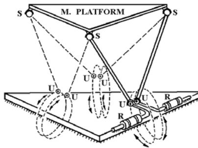
Figure 1. The 6-RUS parallel manipulator introduced by Hunt
