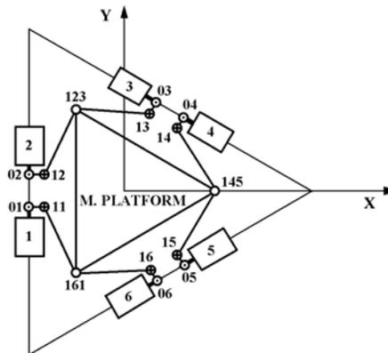
Figure 2. Notation used to describe the parallel manipulator
