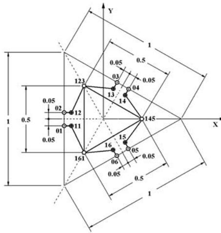
Figure 3. Example of 6-RUS parallel manipulator
